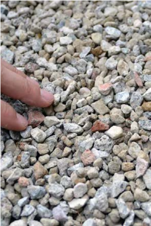
ÁRIDO RECICLADO PARA FORMULACIÓN ECO-GREY® RECYCLED AGGREGATE FOR ECO-GREY® FORMULATION
